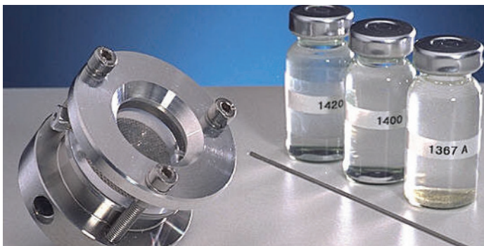
Figure 4: MVTR permeation cell with calibration salt solutions
