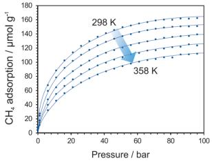
Methane adsorption by a shale
