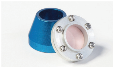
The unique permeation cell for moisture vapor transmission rate (MVTR) determination through membranes.
