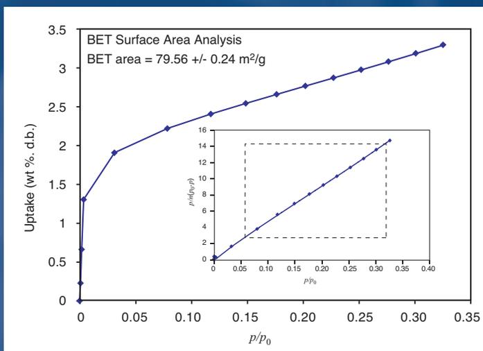
**Figure 6** BET analysis of the specific surface area of the BAM-PM-104 Standard Reference Material measured on an **IMI-PSI**, using nitrogen adsorption at 77 K. The inset shows the BET plot, with the fit performed using the relative pressure range,  $p/p_0 = 0.08$  to  $0.3$
