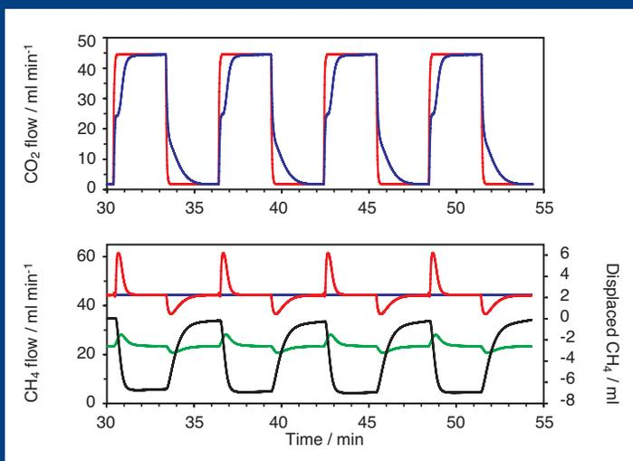
**Figure 9** Dynamic flow experiment designed to determine the nature of selective adsorption of CO<sub>2</sub> over CH<sub>4</sub>. The inlet and outlet CO<sub>2</sub> flows are shown above, while CH<sub>4</sub> flow/displacement and temperature are shown below. See Hiden Isochema Application Note 129 for more information
