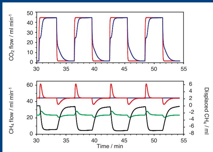
**Figure 9** Dynamic flow experiment designed to determine the nature of selective adsorption of CO<sub>2</sub> over CH<sub>4</sub>. The inlet and outlet CO<sub>2</sub> flows are shown above, while CH<sub>4</sub> flow/displacement and temperature are shown below. See Hiden Isochema Application Note 129 for more information
