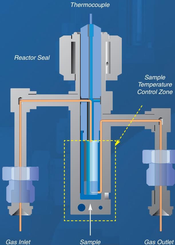
**Figure 3** A layout drawing of the standard IMI reactor, indicating the reactor gas flow path for dynamic (flow) experiments
