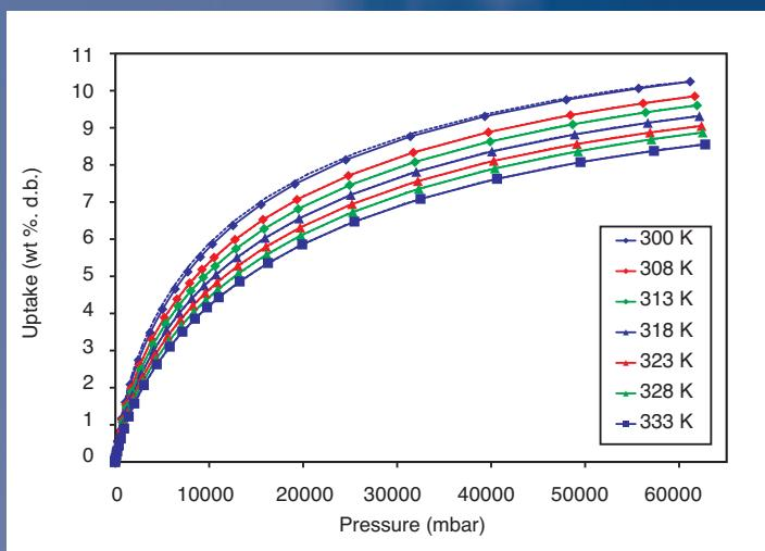
**Figure 7** Reversible methane sorption isotherms measured on a commercial activated carbon (Filtasorb F-400) in an **IMI-NRG** with a large sample reactor between room temperature and 333 K. Adsorption is shown with a solid line while desorption is dashed
