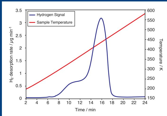
**Figure 8** A thermal desorption (TPD) spectrum showing the amount of hydrogen released from a 3 mg Pd sample hydrogenated in-situ at an elevated temperature and pressure in an **IMI-FLOW**. The hydrogen signal was determined using an optional dynamic sampling mass spectrometer
