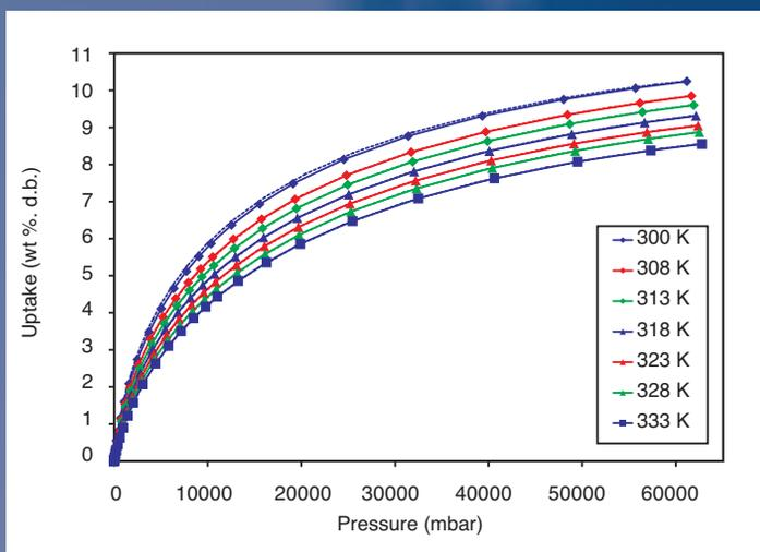
**Figure 7** Reversible methane sorption isotherms measured on a commercial activated carbon (Filtrisorb F-400) in an **IMI-NRG** with a large sample reactor between room temperature and 333 K. Adsorption is shown with a solid line while desorption is dashed
