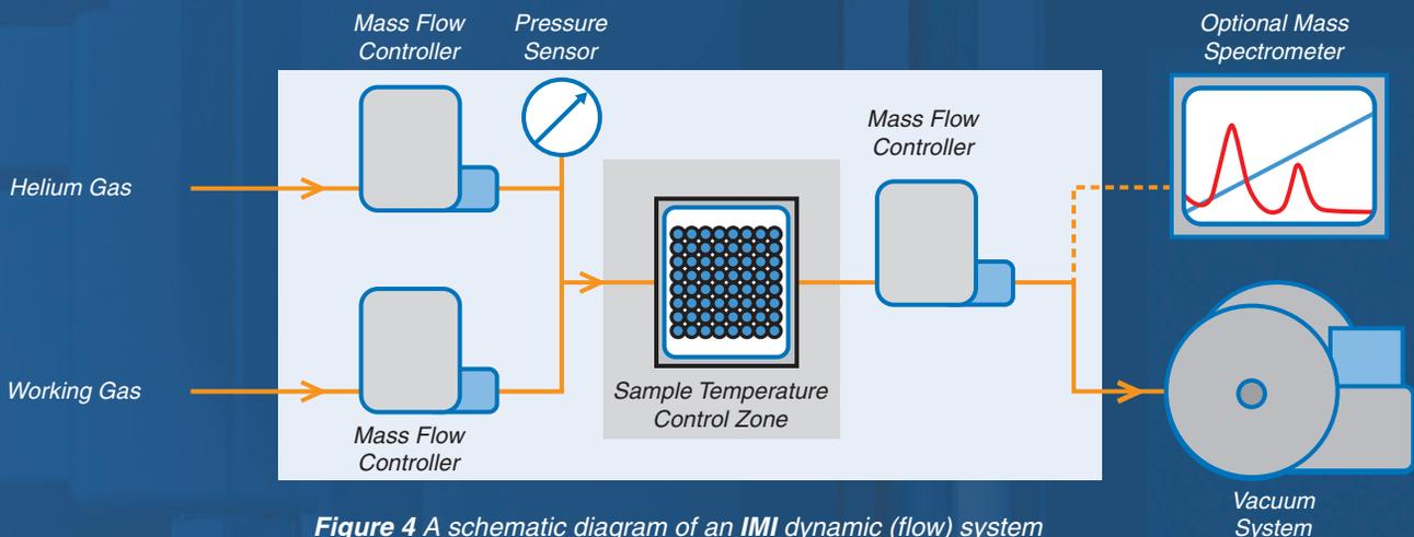
**Figure 4** A schematic diagram of an IMI dynamic (flow) system
