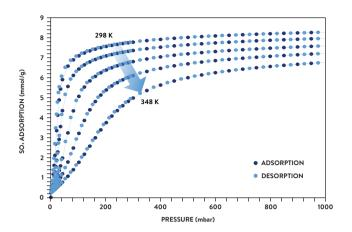
**Figure 1:** SO<sub>2</sub> adsorption by a metal-organic framework (NOTT-300), with kind permission from University of Nottingham, UK.
