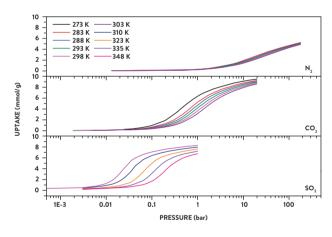
**Figure 4:** N<sub>2</sub>, CO<sub>2</sub> and SO<sub>2</sub> adsorption isotherms on MFM-300(In) over a range of temperatures and pressures. Reproduced with permission from John Wiley and Sons.
