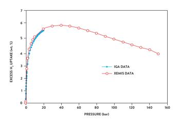
**Figure 3:** Excess H<sub>2</sub> uptake for a 22 mg carbon nanotube, CN4800, using both IGA-003 and XEMIS gravimetric sorption analyzers. Reproduced with permission of The Royal Society of Chemistry.
