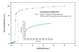
**Figure 6:** Dimethylformamide (DMF) adsorption by a metal-organic framework (MOF), with an inset showing a single step kinetic. Data courtesy of Newcastle University, UK.
