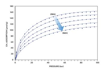
Figure 2: CH<sub>4</sub> adsorption by a shale over a range of temperatures.
