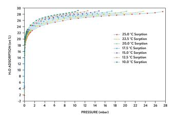
Figure 5: H<sub>2</sub>O adsorption on zeolite 13X powder.
